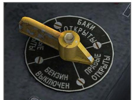
fuel system and allows no fuel to pass beyond the selector valve. The fuel selector is rotating clockwise with left click and anticlockwise with right click.
